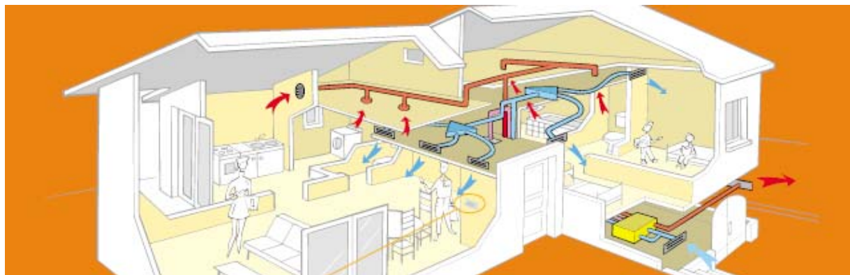
Figure 1-8: Balanced double flow ventilation unit, Courtesy Swedish manufacturers
